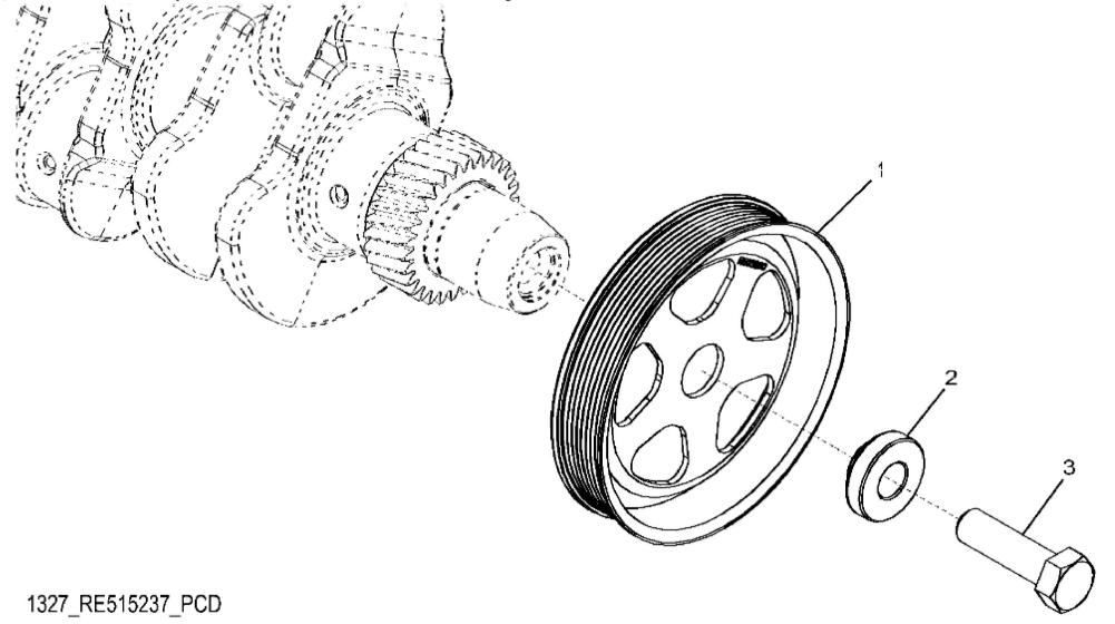
John Deere > Turf And Utility >TRACTOR >5E-854 - TRACTOR >5E-854 Tractor (Stage III)(China Edition\_PIN Prefix 1YR) >20 ENGINE 4045HCP01-RE552170 >ST308624 - 1327 CRANKSHAFT PULLEY
