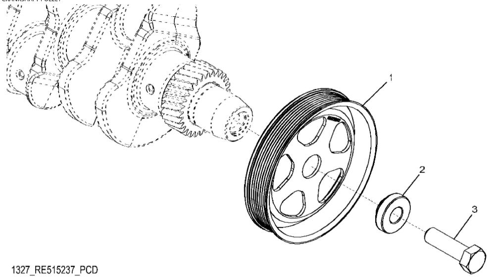
John Deere > Turf And Utility >TRACTOR >5100ML - TRACTOR >5100ML Tractor (Engine 4045HLV68,4045HLV70)(North American Edition) >680 ENGINE 4045HLV68-RE545192 >ST308624 - 1327 CRANKSHAFT PULLEY
