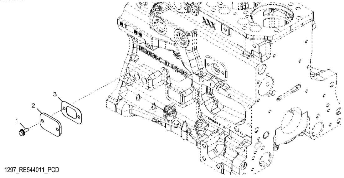
John Deere > Turf And Utility >TRACTOR >5100ML - TRACTOR >5100ML Tractor (Engine 4045HLV68,4045HLV70)(North American Edition) >680 ENGINE 4045HLV68-RE545192 >ST402282 - 1297 OIL FILLER COVER
