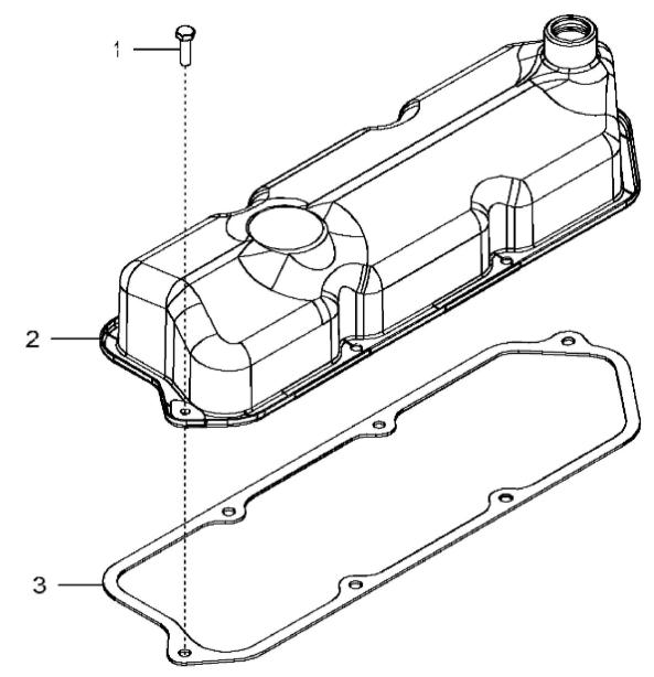
John Deere > Turf And Utility >TRACTOR >5075E - TRACTOR >5075E Tractor (Central Africa, South Africa, Latin America and MENA Edition) >20 ENGINE 3029TPY44-RE565525 METRIC >ST846378 - 1194 ROCKER ARM COVER (XXXXXX - ) John Deere > Turf And Utility >TRACTOR >5075E - TRACTOR >5075E Tractor (Central Africa, South Africa, Latin America and MENA Edition) >20 ENGINE 3029TPY44-RE565525 METRIC >ST846378 - 1194 ROCKER ARM COVER (XXXXXX - )
