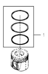
John Deere > Turf And Utility >TRACTOR >5075M - TRACTOR >5075M Tractor (North American Edition)(Engine:3029HYP65)(Final Tier 4) >20 ENGINE 3029HPY65-RE571754 METRIC ( - 000199) >ST833266 - 9901 PISTON RING KIT
