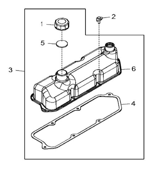
John Deere > Turf And Utility >TRACTOR >5060E - TRACTOR >5060E Tractor (9X3 TSS Transmission W/ Cab)(12X12 PowrReverser Transmission W/ Cab and OOS)(JD Asia and India Edition) >20 ENGINE 3029HPY67-DZ100284 METRIC >ST743365 - 11AB ROCKER ARM COVER
