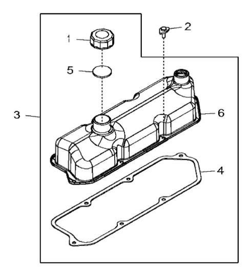
John Deere > Turf And Utility >TRACTOR >5065E - TRACTOR >5065E Tractor (12X12 PowrReverser Transmission W/ Cab and OOS)(JD Asia and India Edition) >20 ENGINE 3029HPY72-DZ100296 METRIC >ST743365 - 11AB ROCKER ARM COVER
