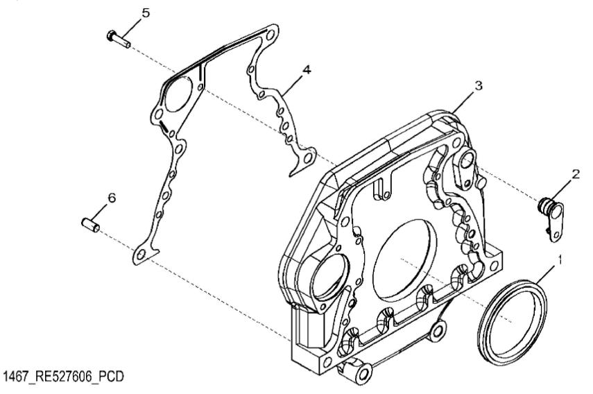
John Deere > Turf And Utility >TRACTOR >5310 - TRACTOR >5310 Tractor (3029HPY59\_RE569735 and 3029HPY60\_RE569736 with TSS Transmission, 3029HPY60\_DZ106808 with PR Transmission)(India Edition) >20 ENGINE 3029HPY59-RE569735 >ST614045 - 1467 FLYWHEEL HOUSING
