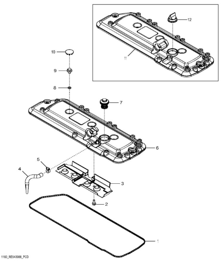
John Deere > Turf And Utility >TRACTOR >5085M - TRACTOR >5085M Tractor (Engine 4045HLV72)(North America Edition)(FT4) >20 ENGINE 4045HLV72-RE565006 >ST400926 - 1183 ROCKER ARM COVER
