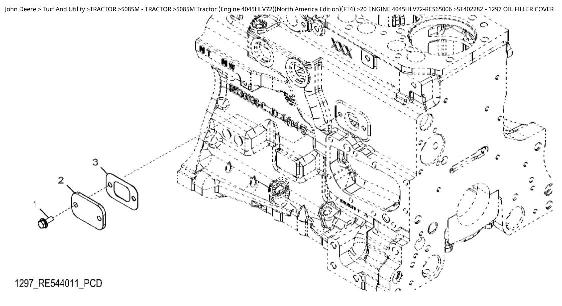
John Deere > Turf And Utility > TRACTOR > 5085M - TRACTOR > 5085M Tractor (Engine 4045HLV72)(North America Edition)(FT4) > 20 ENGINE 4045HLV72-RE565006 > ST402282 - 1297 OIL FILLER COVER
