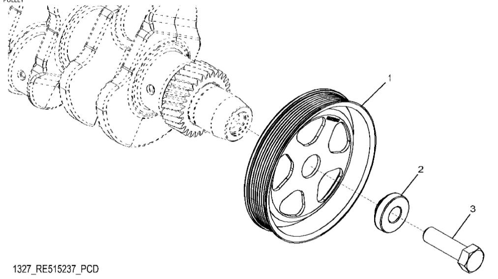
John Deere > Turf And Utility >TRACTOR >5085M - TRACTOR >5085M Tractor (Engine 4045HLV72)(North America Edition)(FT4) >20 ENGINE 4045HLV72-RE565006 >ST308624 - 1327 CRANKSHAFT PULLEY
