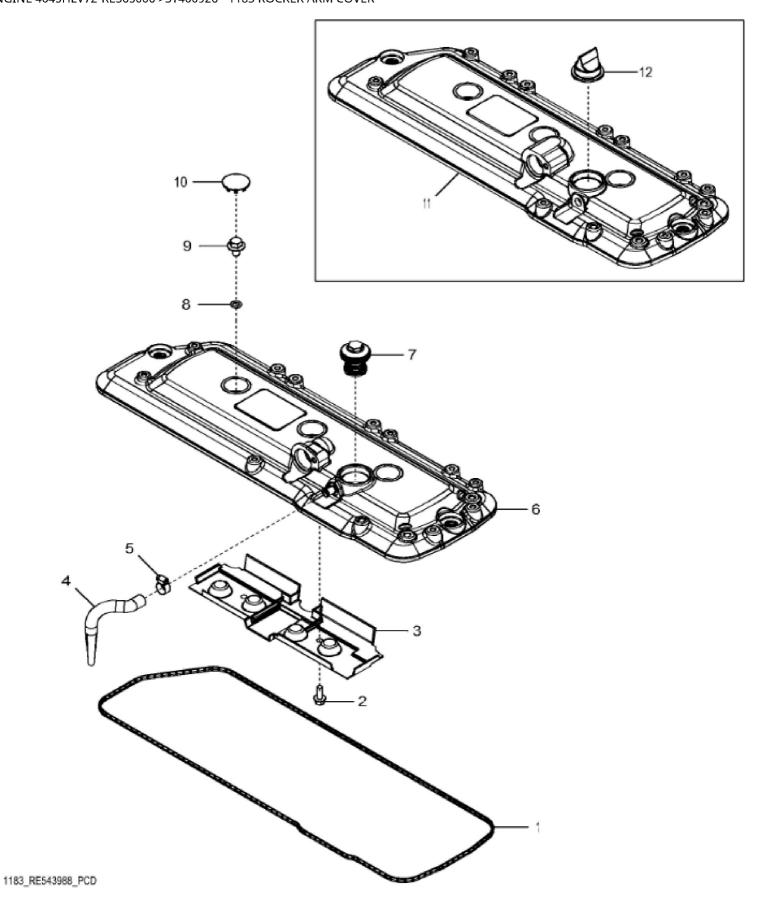
John Deere > Turf And Utility >TRACTOR >5100M - TRACTOR >5100M Tractor (Engine 4045HLV72)(North American Edition)(FT4) >20 ENGINE 4045HLV72-RE565006 >ST400926 - 1183 ROCKER ARM COVER
