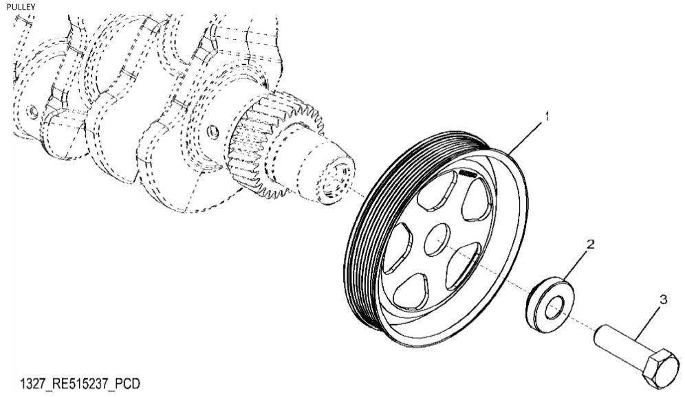
John Deere > Turf And Utility >TRACTOR >5100M - TRACTOR >5100M Tractor (Engine 4045HLV72)(North American Edition)(FT4) >20 ENGINE 4045HLV72-RE565006 >ST308624 - 1327 CRANKSHAFT PULLEY
