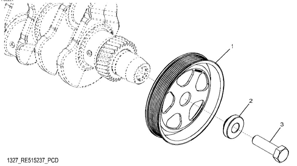
John Deere > Turf And Utility >TRACTOR >5115M - TRACTOR >5115M Tractor (Engine 4045HLV72)(North American Edition)(FT4) >20 ENGINE 4045HLV72-RE565006 >ST308624 - 1327 CRANKSHAFT PULLEY
