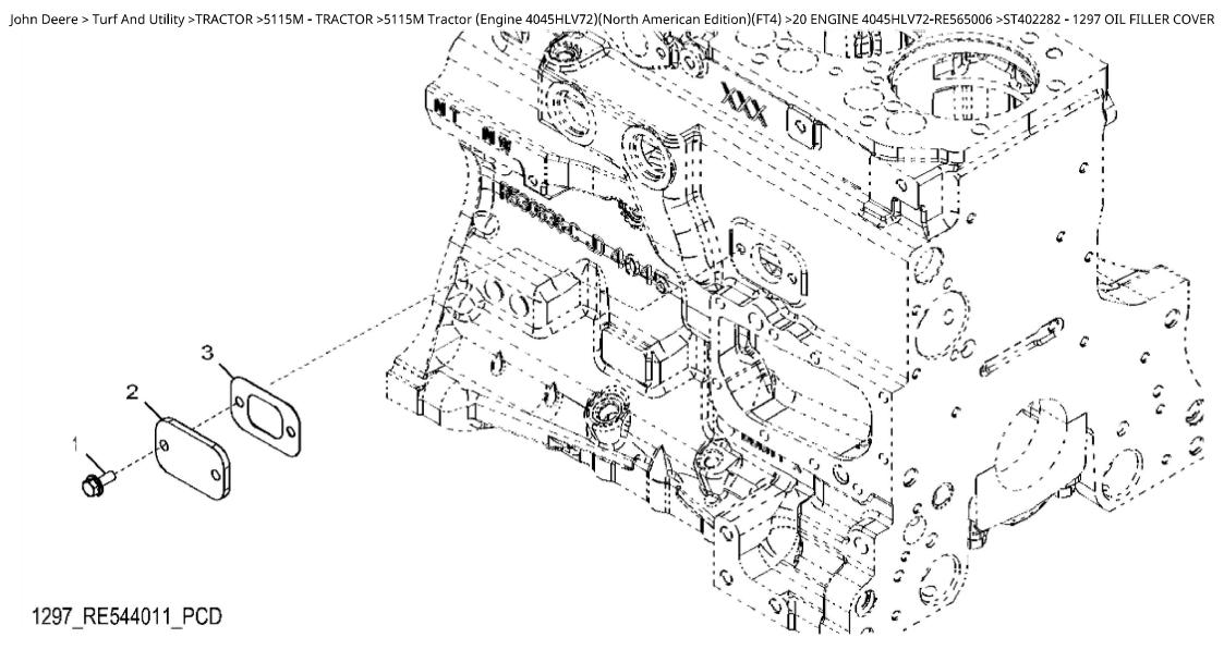
John Deere > Turf And Utility > TRACTOR > 5115M - TRACTOR > 5115M Tractor (Engine 4045HLV72)(North American Edition)(FT4) > 20 ENGINE 4045HLV72-RE565006 > ST402282 - 1297 OIL FILLER COVER
