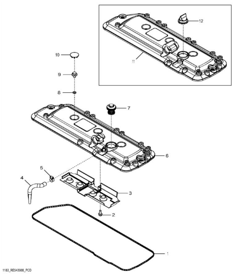
John Deere > Turf And Utility >TRACTOR >5115M - TRACTOR >5115M Tractor (Engine 4045HLV72)(North American Edition)(FT4) >20 ENGINE 4045HLV72-RE565006 >ST400926 - 1183 ROCKER ARM COVER
