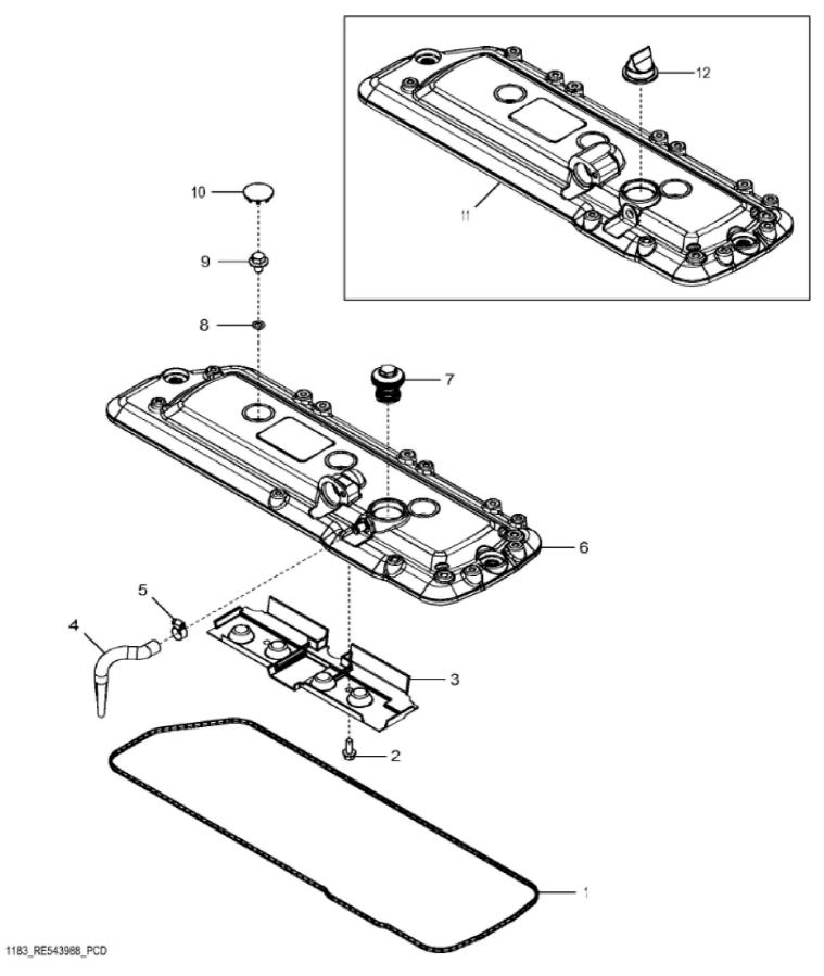
John Deere > Turf And Utility >TRACTOR >5100MH - TRACTOR >5100MH Tractor (Engine 4045HLV72)(North American Edition)(FT4) >20 ENGINE 4045HLV72-RE565006 >ST400926 - 1183 ROCKER ARM COVER
