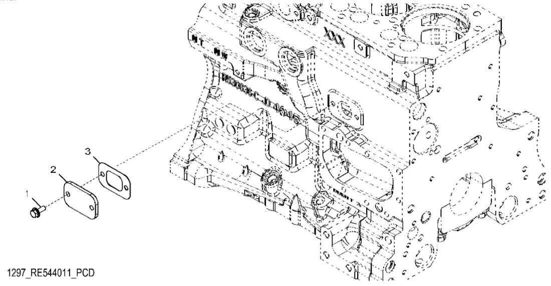
John Deere > Turf And Utility >TRACTOR >5100MH - TRACTOR >5100MH Tractor (Engine 4045HLV72)(North American Edition)(FT4) >20 ENGINE 4045HLV72-RE565006 >ST402282 - 1297 OIL FILLER COVER
