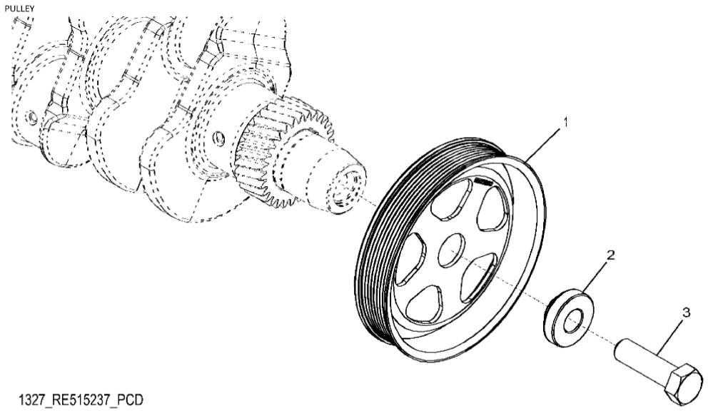
John Deere > Turf And Utility >TRACTOR >5100MH - TRACTOR >5100MH Tractor (Engine 4045HLV72)(North American Edition)(FT4) >20 ENGINE 4045HLV72-RE565006 >ST308624 - 1327 CRANKSHAFT PULLEY
