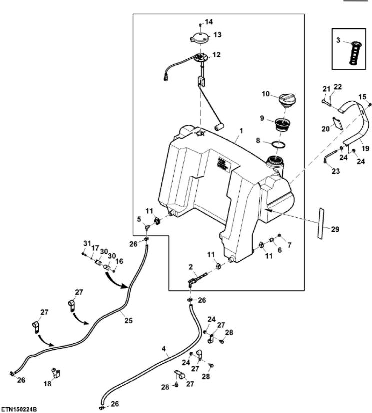
John Deere > Turf And Utility >TRACTOR >554 - TRACTOR >3B-554 Tractor (Stage III) >30 FUEL AND AIR >ST851842 - FUEL TANK, OPTIONAL
