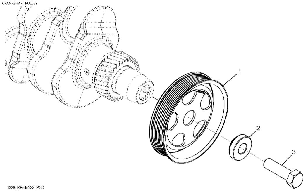
John Deere > Turf And Utility >TRACTOR >5085E - TRACTOR >5085E Tractor (Engine: 4045HLV71, Final Tier 4)(North American Edition) >20 ENGINE 4045HLV71-RE566358 >ST628039 - 1328 CRANKSHAFT PULLEY
