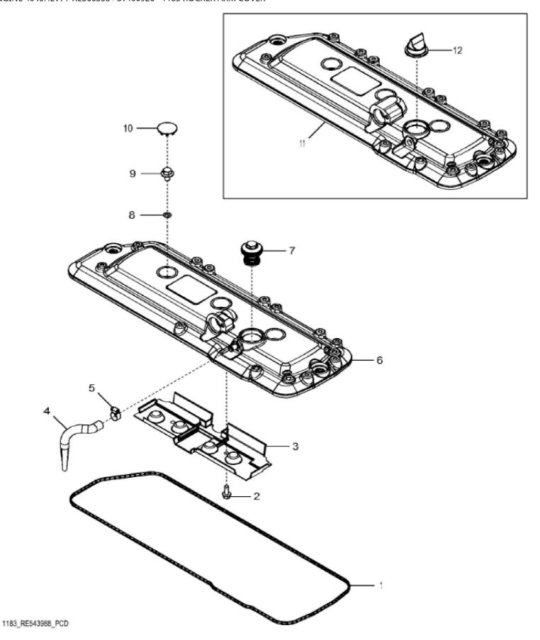
John Deere > Turf And Utility >TRACTOR >5085E - TRACTOR >5085E Tractor (Engine: 4045HLV71, Final Tier 4)(North American Edition) >20 ENGINE 4045HLV71-RE566358 >ST400926 - 1183 ROCKER ARM COVER
