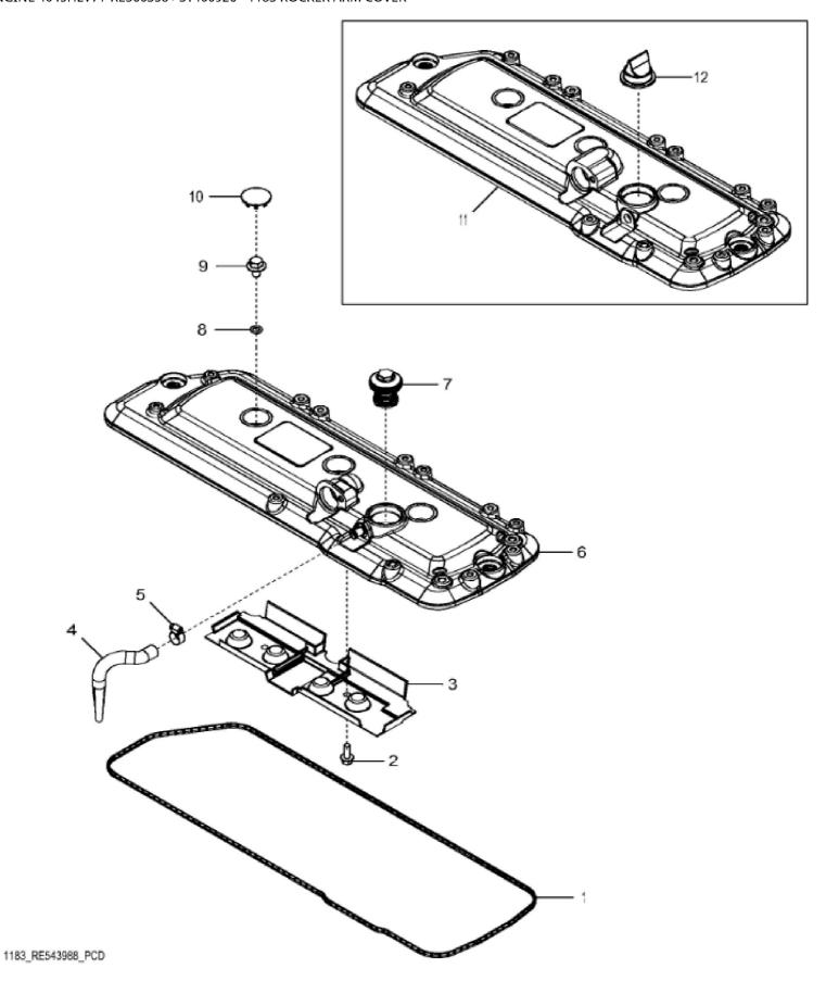
John Deere > Turf And Utility >TRACTOR >5100E - TRACTOR >5100E Tractor (Engine: 4045HLV71, Final Tier 4)(North American Edition) >20 ENGINE 4045HLV71-RE566358 >ST400926 - 1183 ROCKER ARM COVER
