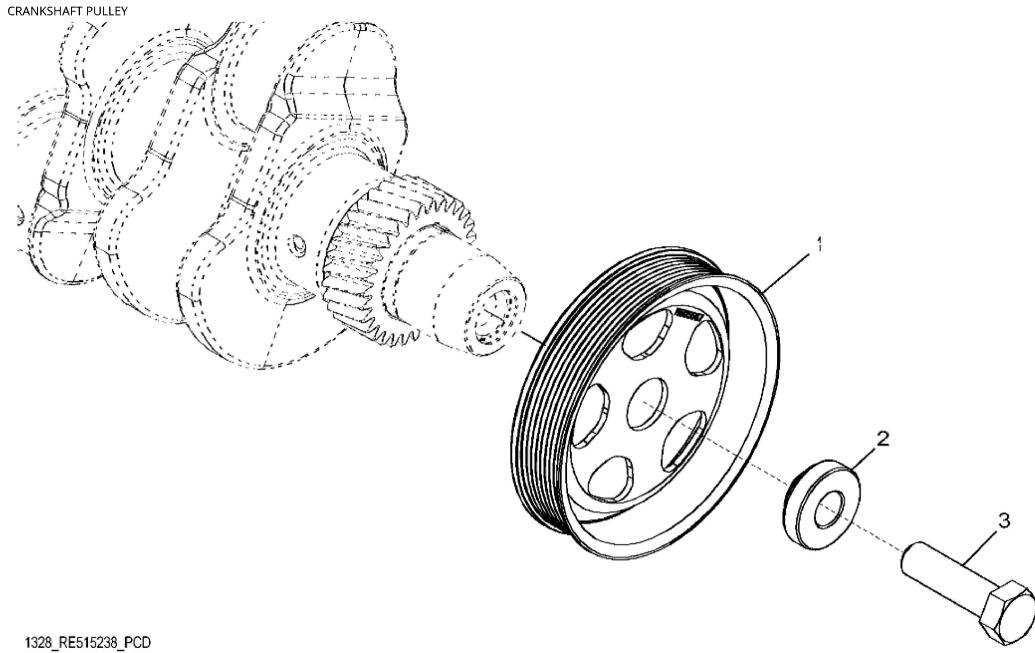
John Deere > Turf And Utility >TRACTOR >5100E - TRACTOR >5100E Tractor (Engine: 4045HLV71, Final Tier 4)(North American Edition) >20 ENGINE 4045HLV71-RE566358 >ST628039 - 1328 CRANKSHAFT PULLEY
