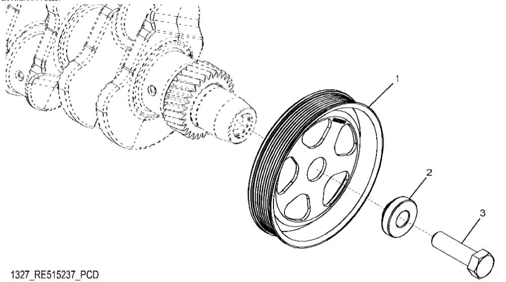
John Deere > Turf And Utility >TRACTOR >5100ML - TRACTOR >5100ML Tractor (Engine 4045HLV72, Final Tier 4)(North American Edition) >20 ENGINE 4045HLV72-RE565006 >ST308624 - 1327 CRANKSHAFT PULLEY
