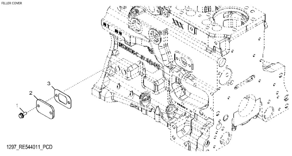
John Deere > Turf And Utility >TRACTOR >5115ML - TRACTOR >5115ML Tractor (Engine 4045HLV72, Final Tier 4)(North America Edition) >20 ENGINE 4045HLV72-RE565006 >ST402282 - 1297 OIL FILLER COVER
