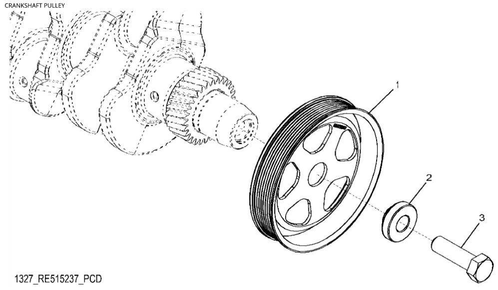
John Deere > Turf And Utility >TRACTOR >5115ML - TRACTOR >5115ML Tractor (Engine 4045HLV72, Final Tier 4)(North America Edition) >20 ENGINE 4045HLV72-RE565006 >ST308624 - 1327 CRANKSHAFT PULLEY
