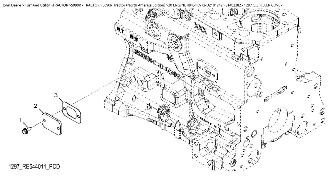
John Deere > Turf And Utility >TRACTOR >5090R - TRACTOR >5090R Tractor (North America Edition) >20 ENGINE 4045HLV73-DZ101242 >ST402282 - 1297 OIL FILLER COVER
