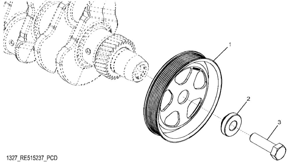
John Deere > Turf And Utility >TRACTOR >5090R - TRACTOR >5090R Tractor (North America Edition) >20 ENGINE 4045HLV73-DZ101242 >ST308624 - 1327 CRANKSHAFT PULLEY
