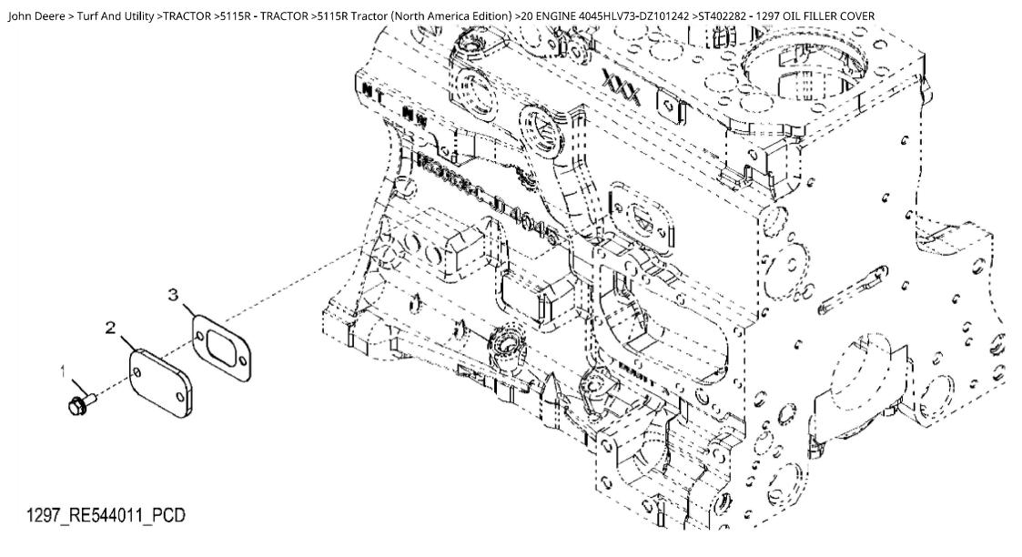
John Deere > Turf And Utility >TRACTOR >5115R - TRACTOR >5115R Tractor (North America Edition) >20 ENGINE 4045HLV73-DZ101242 >ST402282 - 1297 OIL FILLER COVER
