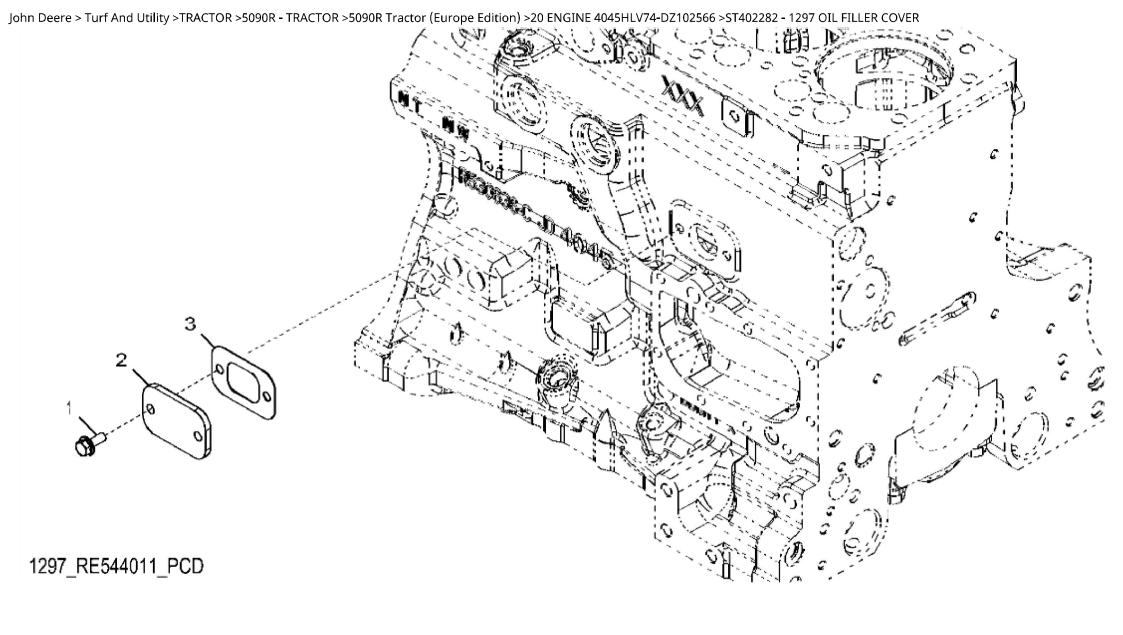
John Deere > Turf And Utility >TRACTOR >5090R - TRACTOR >5090R Tractor (Europe Edition) >20 ENGINE 4045HLV74-DZ102566 >ST402282 - 1297 OIL FILLER COVER
