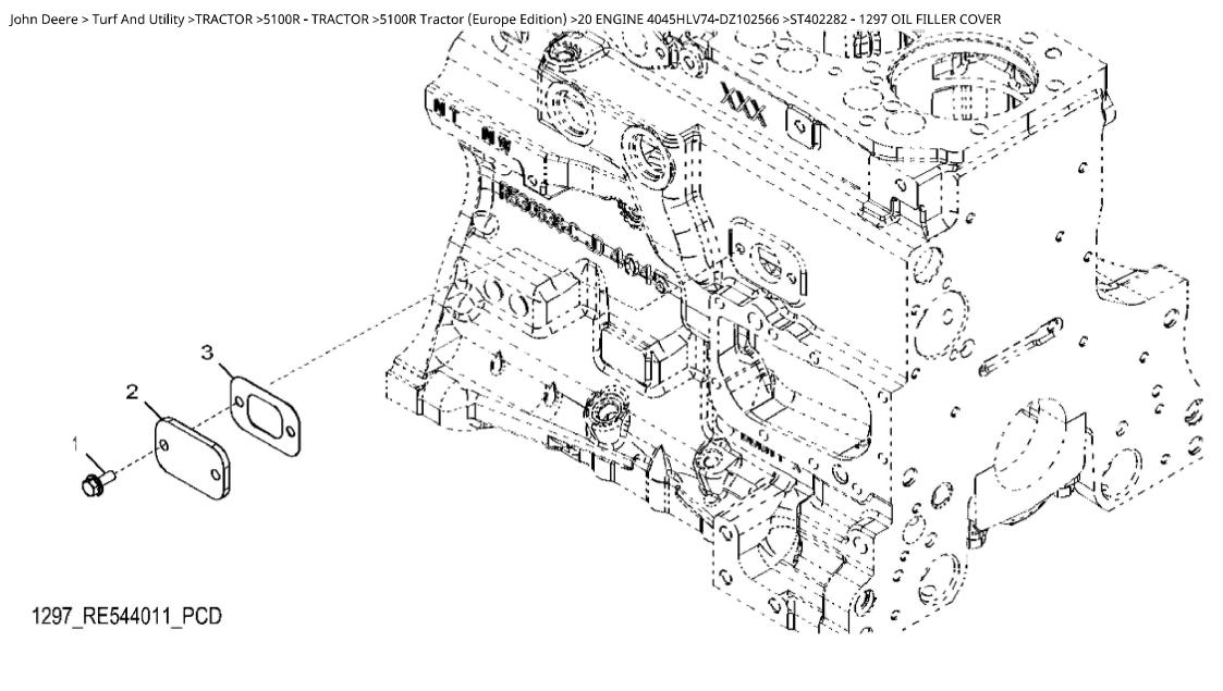
John Deere > Turf And Utility >TRACTOR >5100R - TRACTOR >5100R Tractor (Europe Edition) >20 ENGINE 4045HLV74-DZ102566 >ST402282 - 1297 OIL FILLER COVER
