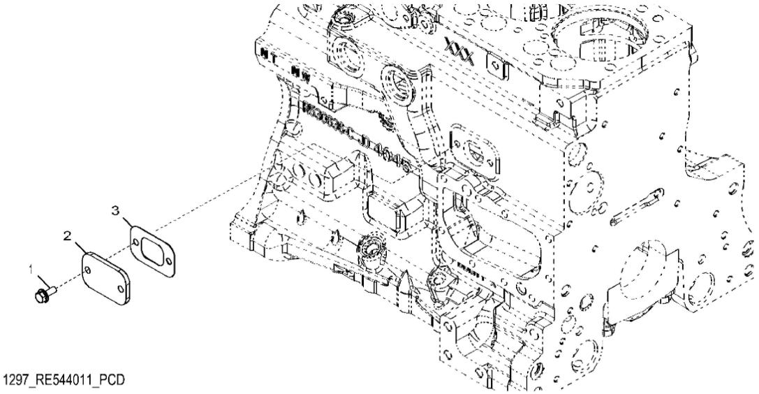
John Deere > Turf And Utility >TRACTOR >6130M - TRACTOR >6130M Tractor (Europe Edition, Engine SN: 4045UXXXXXX)(Final Tier 4) >E1 ENGINE 4045HL500-DD22292-ETN122284-ETN122286-ETN131686 +045HL500 >ST402282 - 1297 OIL FILLER COVER
