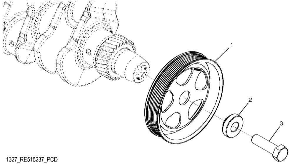
John Deere > Turf And Utility >TRACTOR >6135M - TRACTOR >6135M Tractor (Europe Edition, Engine SN: 4045UXXXXX)(Final Tier 4) >E1 ENGINE 4045HL501-DD22310-ETN124754-ETN131687 >E100 ENGINE 4045HL501-DD22310-ETN124754-ETN131687 4045HL501 >ST308624 - 1327 CRANKSHAFT PULLEY
