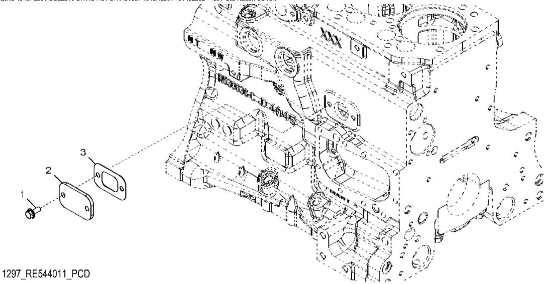
John Deere > Turf And Utility >TRACTOR >6135M - TRACTOR >6135M Tractor (Europe Edition, Engine SN: 4045UXXXXX)(Final Tier 4) >E1 ENGINE 4045HL501-DD22310-ETN124754-ETN131687 +E100 ENGINE 4045HL501-DD22310-ETN124754-ETN131687 +E102282 - 1297 OIL FILLER COVER
