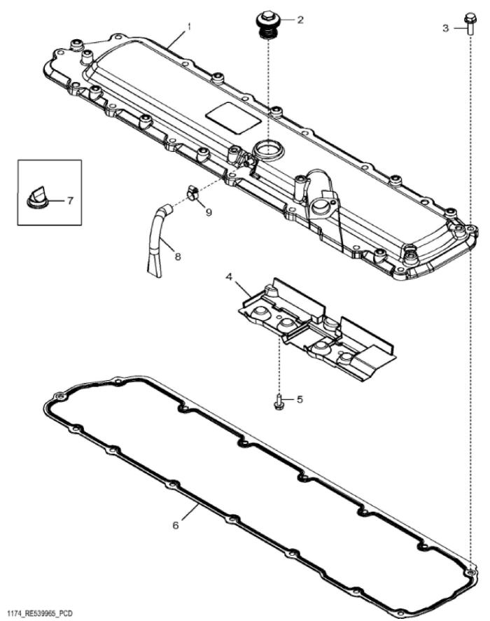
John Deere > Turf And Utility >TRACTOR >6155M - TRACTOR >6155M Tractor (Europe Edition, Engine SN: 6068UXXXXXX)(Final Tier 4) >E1 DIESEL ENGINE 6068HL498-DD22386-ETN122786-ETN122787-ETN131688 6068HL498 >ST164694 - 1174 ROCKER ARM COVER
