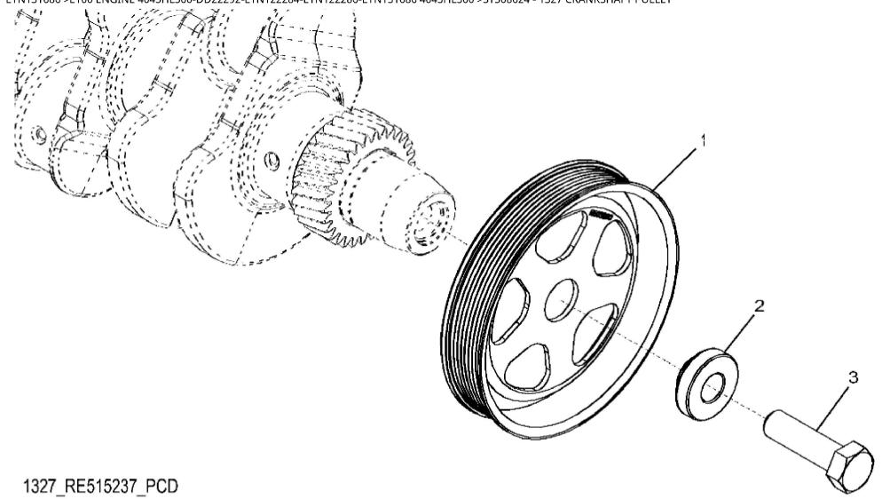
John Deere > Turf And Utility > TRACTOR > 6110M - TRACTOR > 6110M Tractor (North America Edition, Engine SN: 4045UXXXXXX)(Final Tier 4) > E1 ENGINE 4045HL500-DD22292-ETN122284-ETN122286-ETN131686 > E100 ENGINE 4045HL500-DD22292-ETN122284-ETN122286-ETN131686 4045HL500 > ST308624 - 1327 CRANKSHAFT PULLEY
