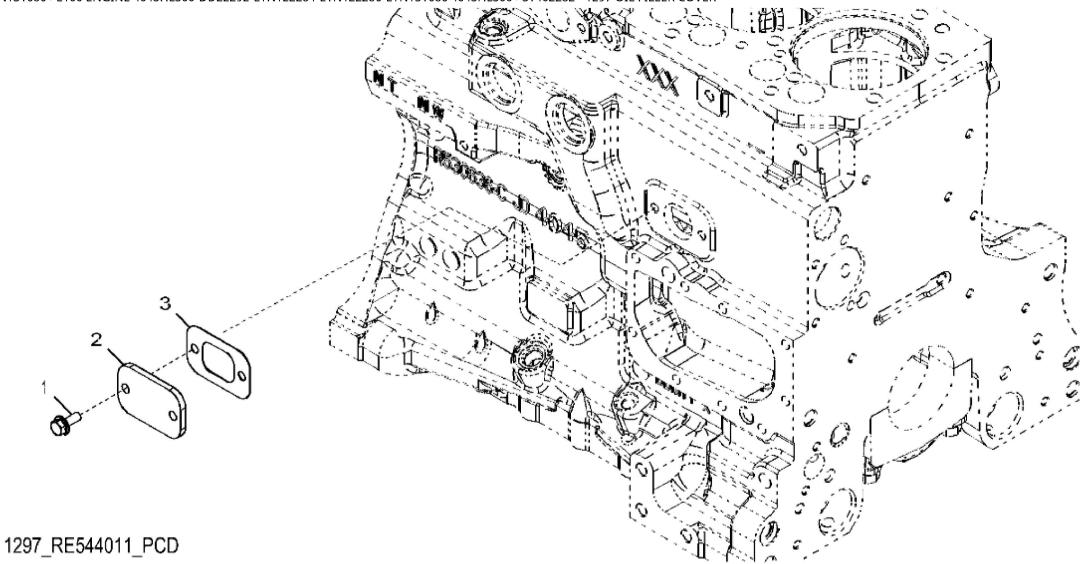
John Deere > Turf And Utility >TRACTOR >6130M - TRACTOR >6130M Tractor (North America Edition, Engine SN: 4045UXXXXX)(Final Tier 4) >E1 ENGINE 4045HL500-DD22292-ETN122284-ETN122286-ETN131686 4045HL500 >ST402282 - 1297 OIL FILLER COVER
