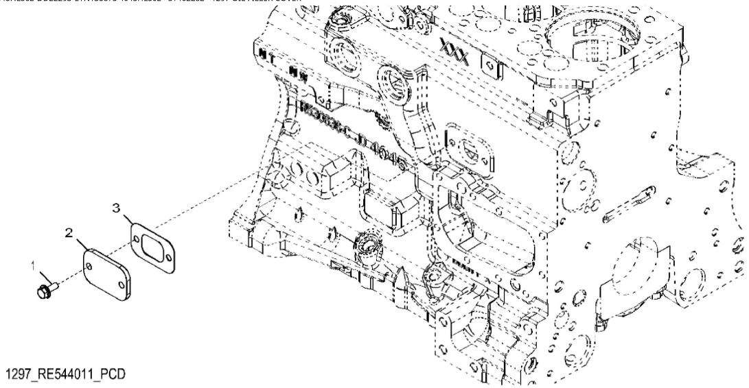
John Deere > Turf And Utility >TRACTOR >6095MC - TRACTOR >6095MC Tractor (Europe Edition, Engine SN: 4045UXXXXXX)(Final Tier 4) >EN ENGINE 4045HL502-DD22293-ETN135873 >EN00 ENGINE 4045HL502-DD22293-ETN135873 4045HL502 >ST402282 - 1297 OIL FILLER COVER
