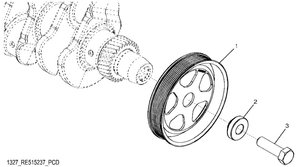
John Deere > Turf And Utility >TRACTOR >6095MC - TRACTOR >6095MC Tractor (Europe Edition, Engine SN: 4045UXXXXXX)(Final Tier 4) >EN ENGINE 4045HL502-DD22293-ETN135873 >EN00 ENGINE 4045HL502-DD22293-ETN135873 4045HL502 >ST308624 - 1327 CRANKSHAFT PULLEY
