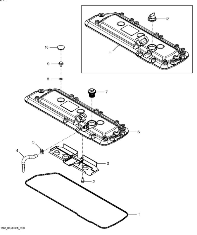
John Deere > Turf And Utility >TRACTOR >6115MC - TRACTOR >6115MC Tractor (Europe Edition, Engine SN: 4045UXXXXXX)(Final Tier 4) >EN ENGINE 4045HL502-DD22293-ETN135873 >EN00 ENGINE 4045HL502-DD22293-ETN135873 4045HL502 >ST400926 - 1183 ROCKER ARM COVER
