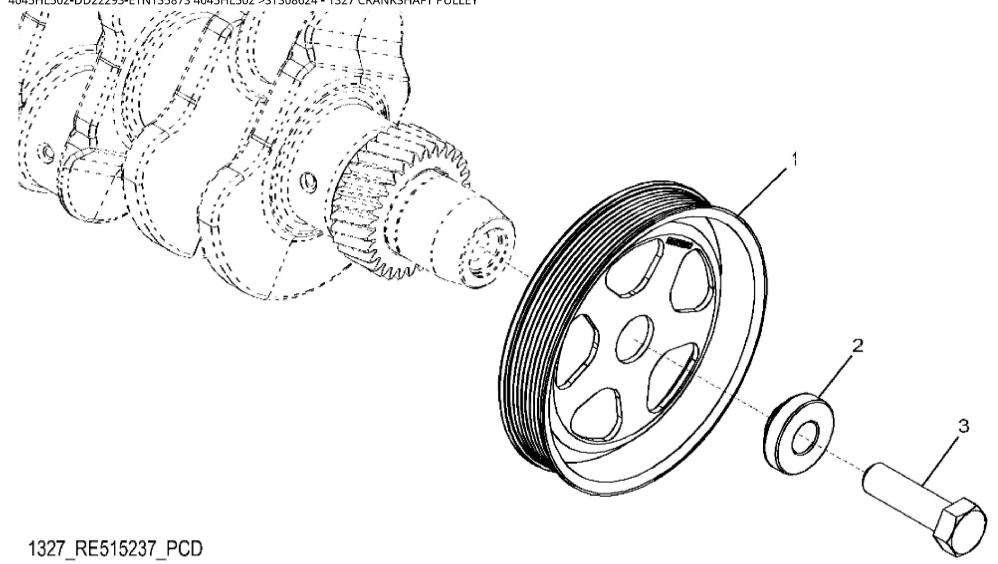
John Deere > Turf And Utility >TRACTOR >6115MC - TRACTOR >6115MC Tractor (Europe Edition, Engine SN: 4045UXXXXXX)(Final Tier 4) >EN ENGINE 4045HL502-DD22293-ETN135873 >EN00 ENGINE 4045HL502-DD22293-ETN135873 4045HL502 >ST308624 - 1327 CRANKSHAFT PULLEY
