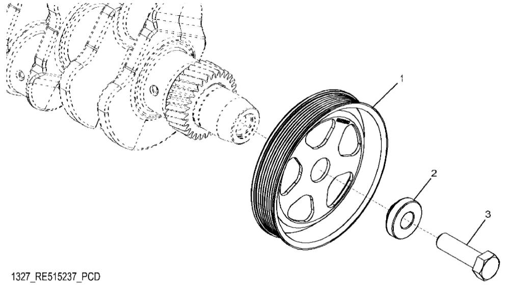
John Deere > Turf And Utility >TRACTOR >6125M - TRACTOR >6125M Tractor (Europe Edition, Engine SN: 4045GXXXXXX)(Tier 2)(S.N. 859738-) >EN ENGINE 4045HL289-DZ105554-ETN150958 >EN00 ENGINE 4045HL289-DZ105554-ETN150958 4045HL289 >ST308624 - 1327 CRANKSHAFT PULLEY
