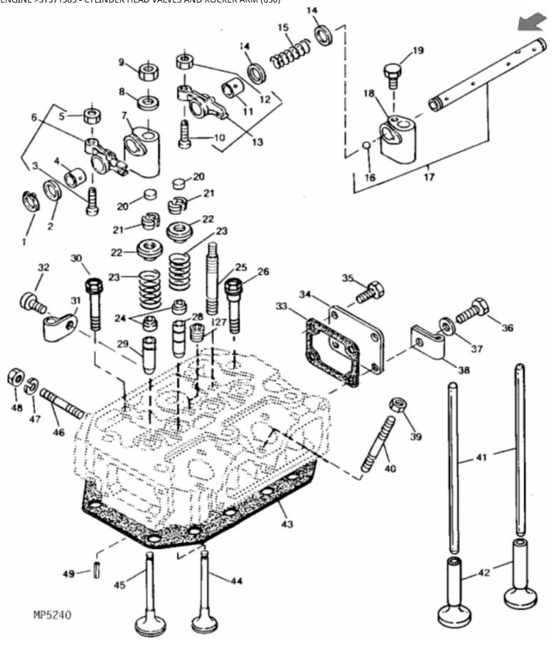
John Deere > Turf And Utility >TRACTOR, COMPACT UTILITY >750 - TRACTOR, COMPACT UTILITY >650 and 750 Compact Utility Tractors >20 ENGINE >ST571385 - CYLINDER HEAD VALVES AND ROCKER ARM (650)
