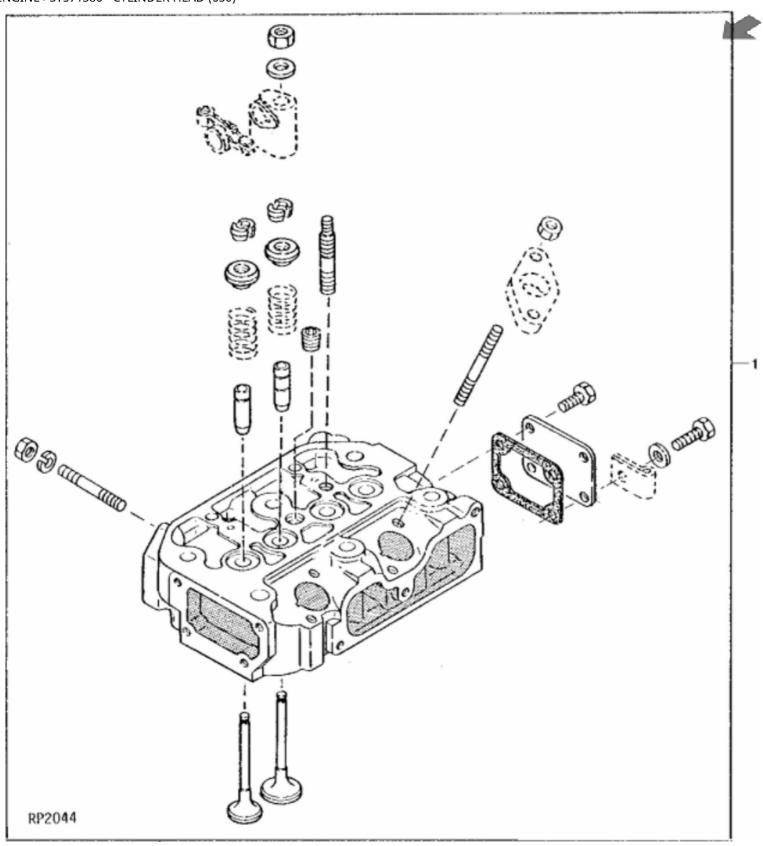
John Deere > Turf And Utility >TRACTOR, COMPACT UTILITY >750 - TRACTOR, COMPACT UTILITY >650 and 750 Compact Utility Tractors >20 ENGINE >ST571386 - CYLINDER HEAD (650)
