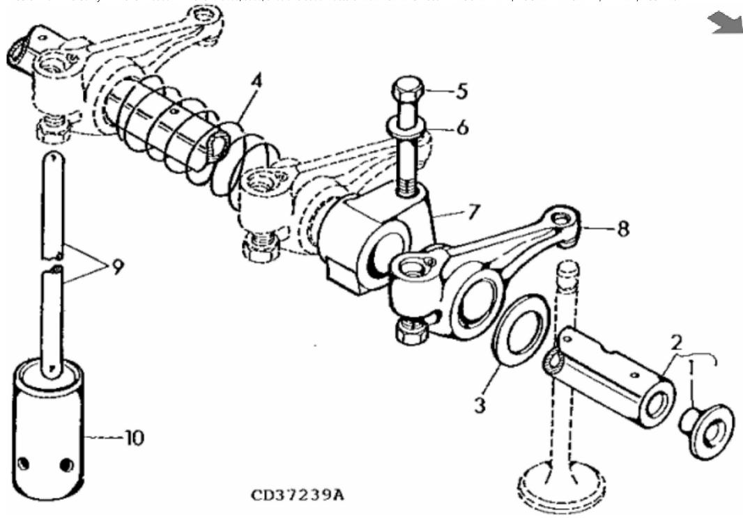
John Deere > Turf And Utility >TRACTOR >5500 - TRACTOR >5200, 5300, 5400 and 5500 Tractors >20 ENGINE >ST435971 - ROCKER ARM / ROCKER ARM SHAFT / TAPPET / PUSH ROD
