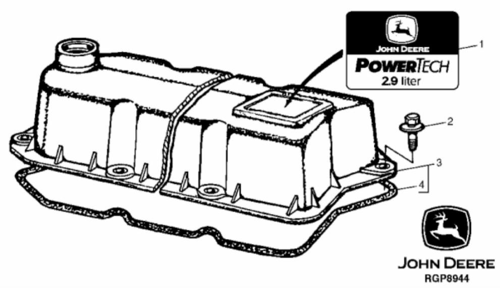
John Deere > Turf And Utility >TRACTOR >5510 - TRACTOR >5210, 5310, 5410 and 5510 Tractors (North America Edition) >20 ENGINE (5210, 5310) >ST437098 - VALVE COVER
