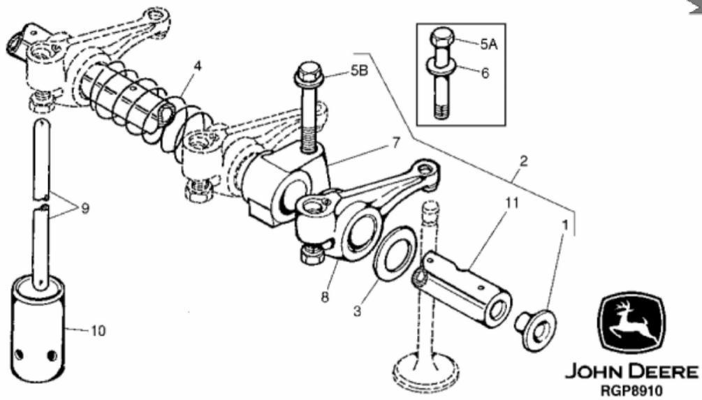
John Deere > Turf And Utility >TRACTOR >5510 - TRACTOR >5210, 5310, 5410 and 5510 Tractors (North America Edition) >20 ENGINE (5210, 5310) >ST437100 - ROCKER ARM SHAFT
