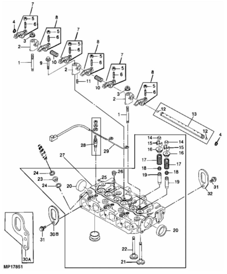
John Deere > Turf And Utility >TRACTOR, COMPACT UTILITY >4100 - TRACTOR, COMPACT UTILITY >4100 Compact Utility Tractor >20 ENGINE >ST638503 - CYLINDER HEAD, VALVES AND ROCKER ARMS
