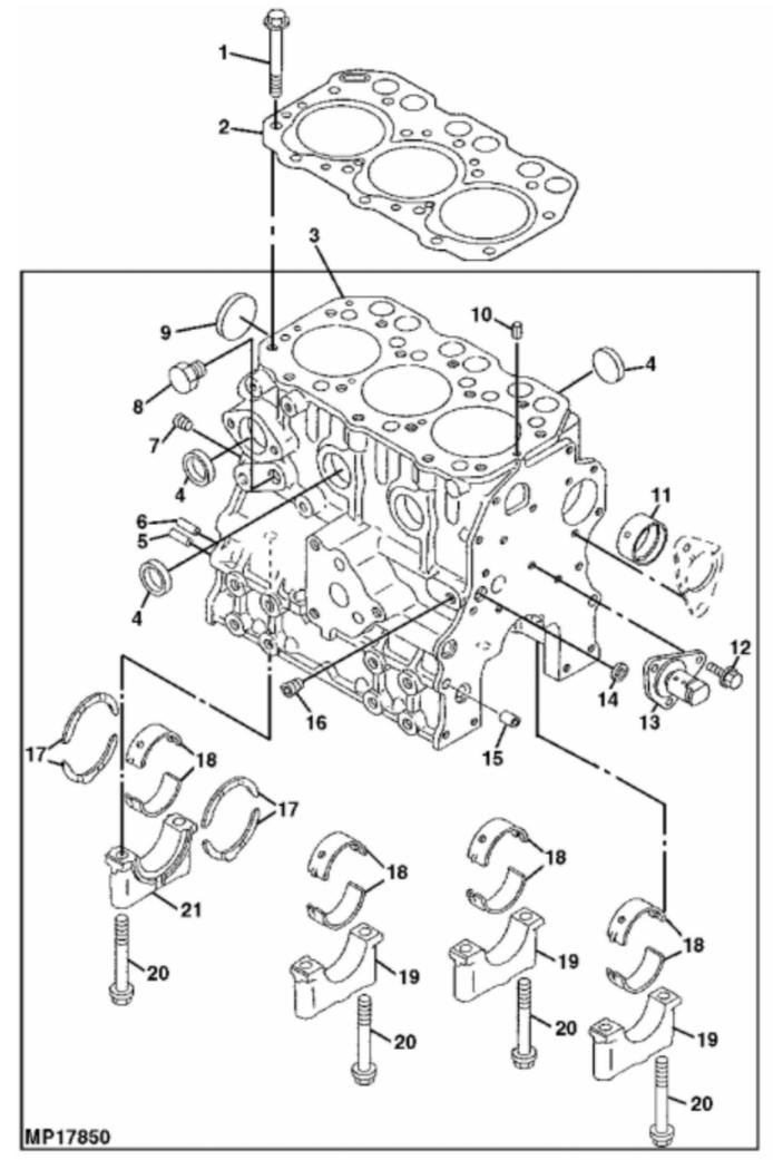
John Deere > Turf And Utility >TRACTOR, COMPACT UTILITY >4100 - TRACTOR, COMPACT UTILITY >4100 Compact Utility Tractor >20 ENGINE >ST638502 - CYLINDER BLOCK AND MAIN BEARINGS
