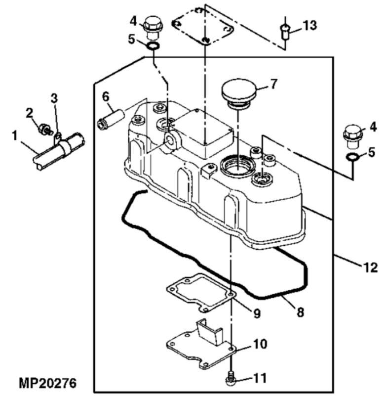
John Deere > Turf And Utility >TRACTOR, COMPACT UTILITY >4100 - TRACTOR, COMPACT UTILITY >4100 Compact Utility Tractor >20 ENGINE >ST638504 - CYLINDER HEAD COVER AND GASKETS
