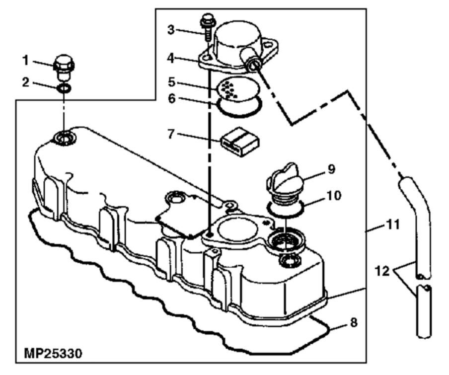
John Deere > Turf And Utility >TRACTOR, COMPACT UTILITY >4500 - TRACTOR, COMPACT UTILITY >4500 Compact Utility Tractors >20 ENGINE >ST633057 - CYLINDER HEAD COVER AND GASKETS
