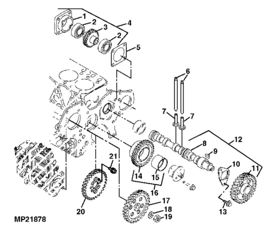
John Deere > Turf And Utility >TRACTOR, COMPACT UTILITY >4500 - TRACTOR, COMPACT UTILITY >4500 Compact Utility Tractors >20 ENGINE >ST638933 - CAMSHAFT AND DRIVING GEARS
