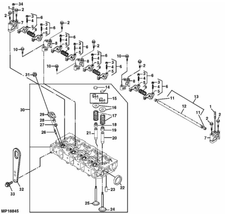
John Deere > Turf And Utility >TRACTOR, COMPACT UTILITY >4500 - TRACTOR, COMPACT UTILITY >4500 Compact Utility Tractors >20 ENGINE >ST638931 - CYLINDER HEAD, VALVES AND ROCKER ARMS
