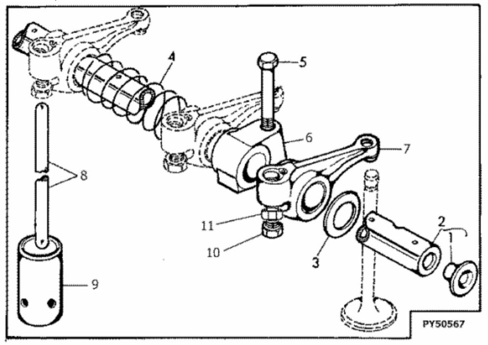
John Deere > Turf And Utility >TRACTOR >5310 - TRACTOR >5310 Tractor (SN -PY5310S005118)(India Edition) >20 ENGINE >20-3 - ROCKER ARM / SHAFT / TAPPET / PUSH ROD [A18]
