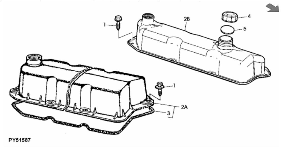
John Deere > Turf And Utility >TRACTOR >5204 - TRACTOR >5103E, 5103, 5103S, 5203, 5104, 5038D (S.N. -009920), 5204 Tractors(India Edition) >20 ENGINE >ST665582 - VALVE COVER
