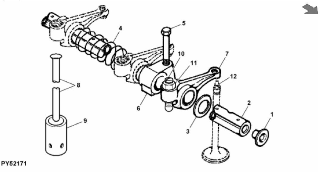
John Deere > Turf And Utility > TRACTOR > 5204 - TRACTOR > 5103E, 5103, 5103S, 5203, 5104, 5038D (S.N. -009920), 5204 Tractors(India Edition) > 20 ENGINE > ST665584 - ROCKER ARM / ROCKER ARM SHAFT / TAPPET / PUSH ROD
