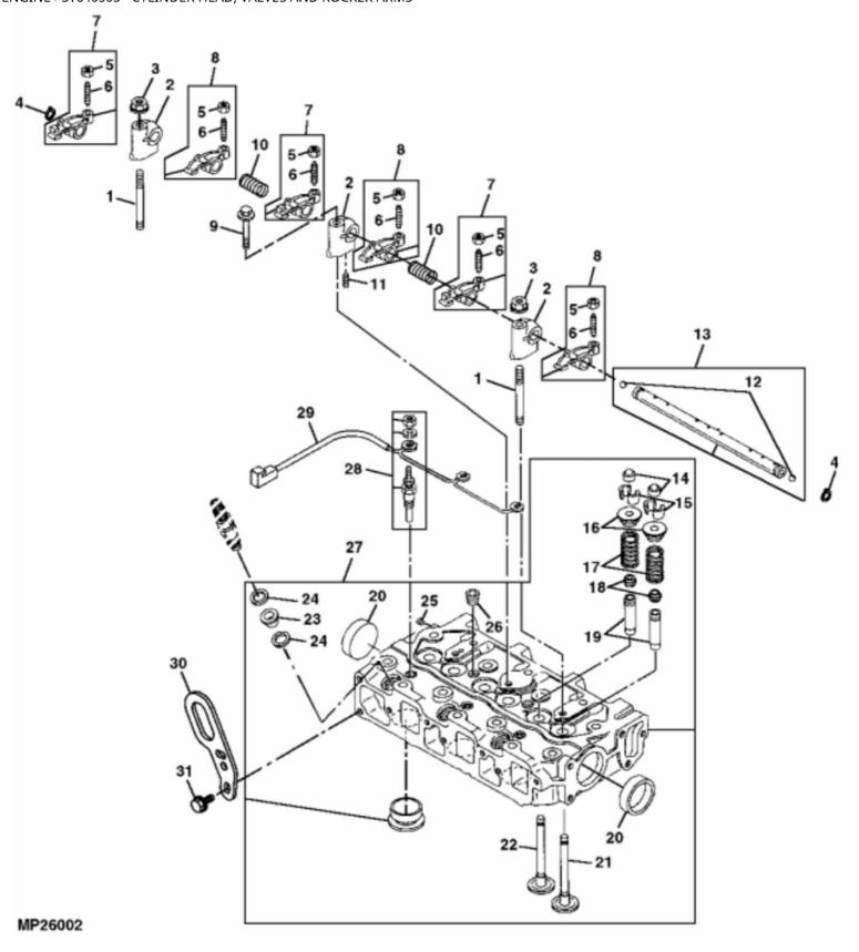
John Deere > Turf And Utility >TRACTOR, COMPACT UTILITY >4010 - TRACTOR, COMPACT UTILITY >4010 Compact Utility Tractor >20 ENGINE >ST640505 - CYLINDER HEAD, VALVES AND ROCKER ARMS
