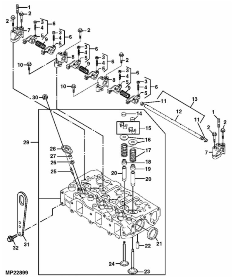
John Deere > Turf And Utility >TRACTOR, COMPACT UTILITY >4115 - TRACTOR, COMPACT UTILITY >4115 Compact Utility Tractor >20 ENGINE >ST640637 - CYLINDER HEAD, VALVES AND ROCKER ARMS
