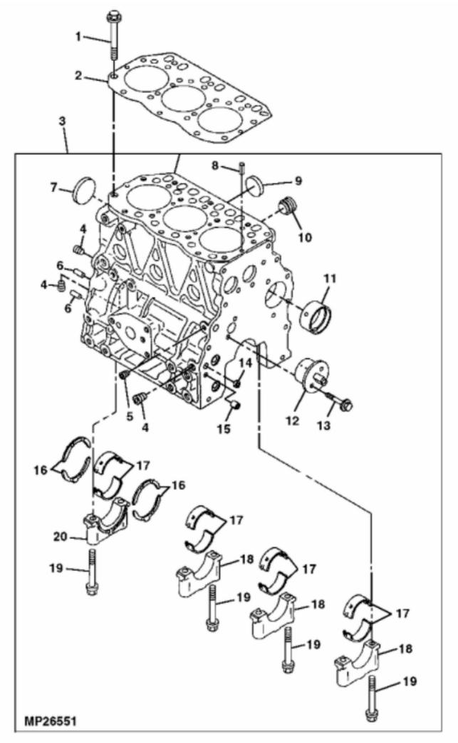
John Deere > Turf And Utility >TRACTOR, COMPACT UTILITY >4115 - TRACTOR, COMPACT UTILITY >4115 Compact Utility Tractor >20 ENGINE >ST640636 - CYLINDER BLOCK AND MAIN BEARINGS
