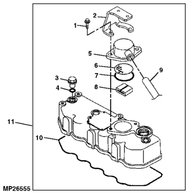
John Deere > Turf And Utility >TRACTOR, COMPACT UTILITY >4115 - TRACTOR, COMPACT UTILITY >4115 Compact Utility Tractor >20 ENGINE >ST640638 - CYLINDER HEAD COVER AND GASKETS
