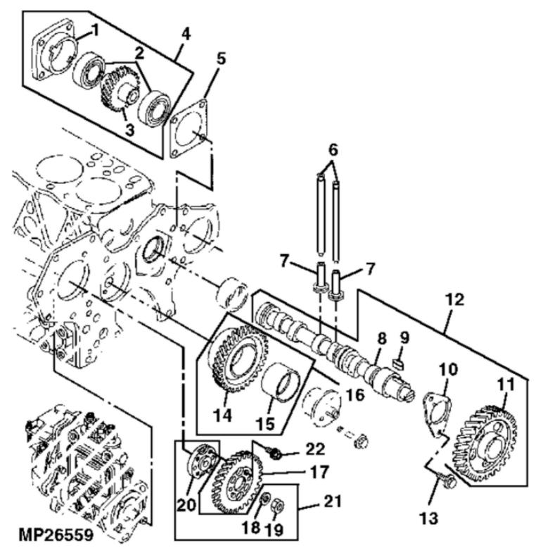
John Deere > Turf And Utility >TRACTOR, COMPACT UTILITY >4115 - TRACTOR, COMPACT UTILITY >4115 Compact Utility Tractor >20 ENGINE >ST640639 - CAMSHAFT AND DRIVING GEARS
