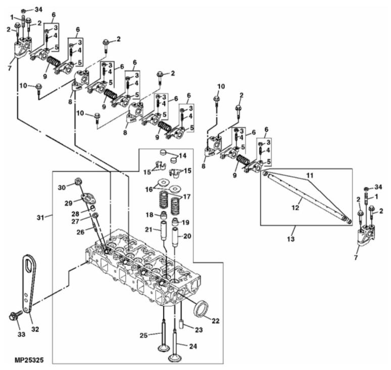
John Deere > Turf And Utility >TRACTOR, COMPACT UTILITY >4710 - TRACTOR, COMPACT UTILITY >4710 Compact Utility Tractor >20 ENGINE >ST643645 - CYLINDER HEAD, VALVES AND ROCKER ARMS
