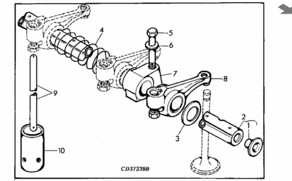
John Deere > Turf And Utility >TRACTOR >5500 - TRACTOR >5300, 5400, 5500 Tractors (Europe Edition) >20 ENGINE CD3029DAT01, CD3029TAT02, CD4039TAT01 >ST115485 - ROCKER ARM / SHAFT / TAPPET / PUSH ROD (DAT01, TAT02) ( - 394178)
