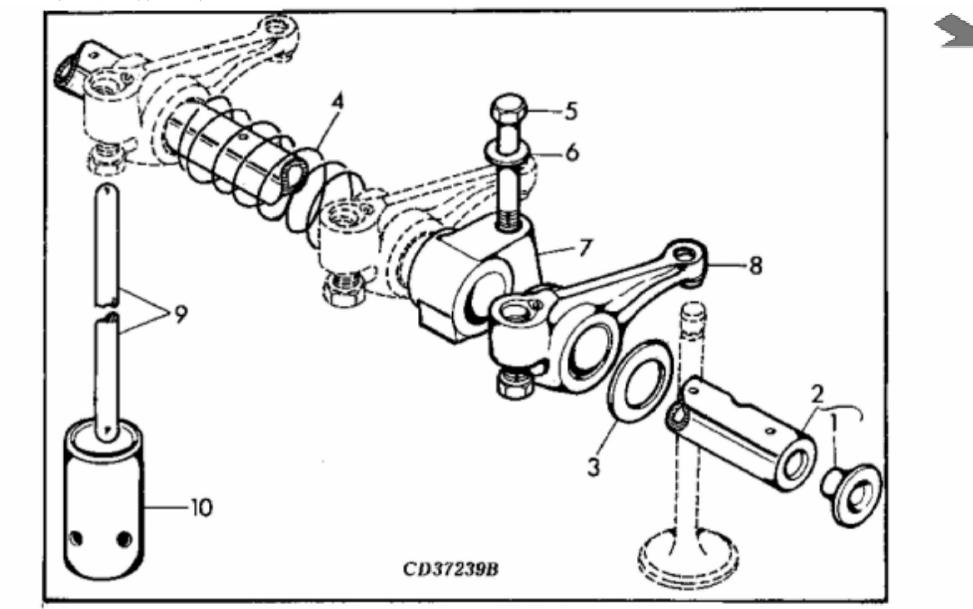
John Deere > Turf And Utility >TRACTOR >5500N - TRACTOR >5300N, 5400N, 5500N Tractors (Europe Edition) >20 ENGINE CD3029DAT01, CD3029TAT02, CD4039TAT01 >ST115485 - ROCKER ARM / SHAFT / TAPPET / PUSH ROD (DAT01, TAT02) ( - 394178)
