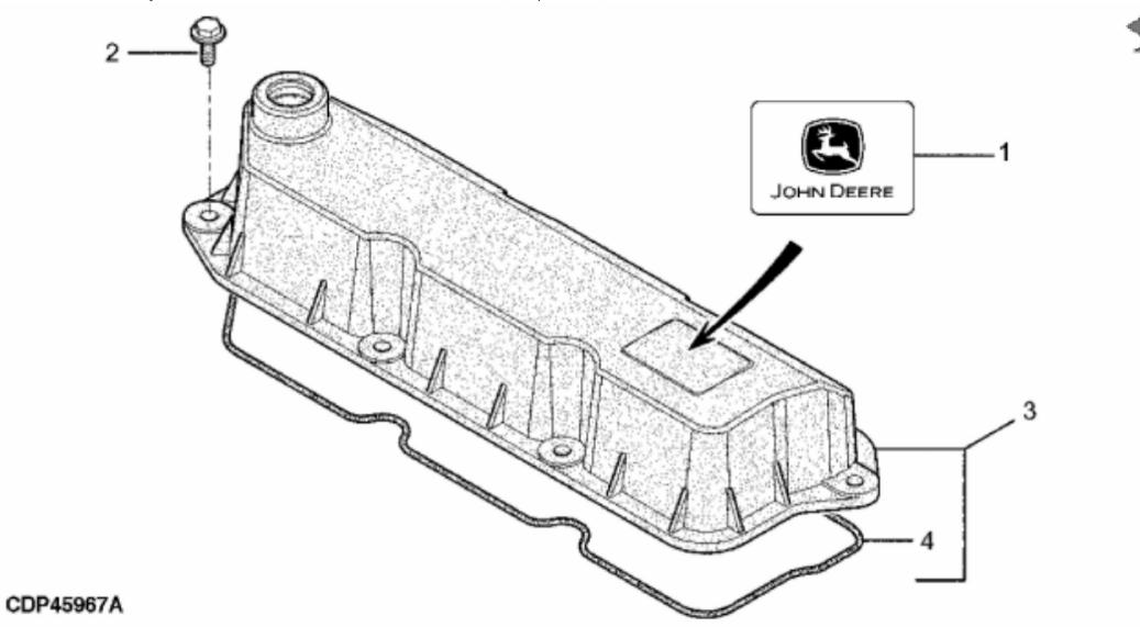
John Deere > Turf And Utility >TRACTOR >5510 - TRACTOR >5310, 5410, 5510 Tractors (Europe Edition) >20 ENGINE 3029DAT50 & 3029TAT50-DD16145 - DD16145 >ST116740 - VALVE COVER
