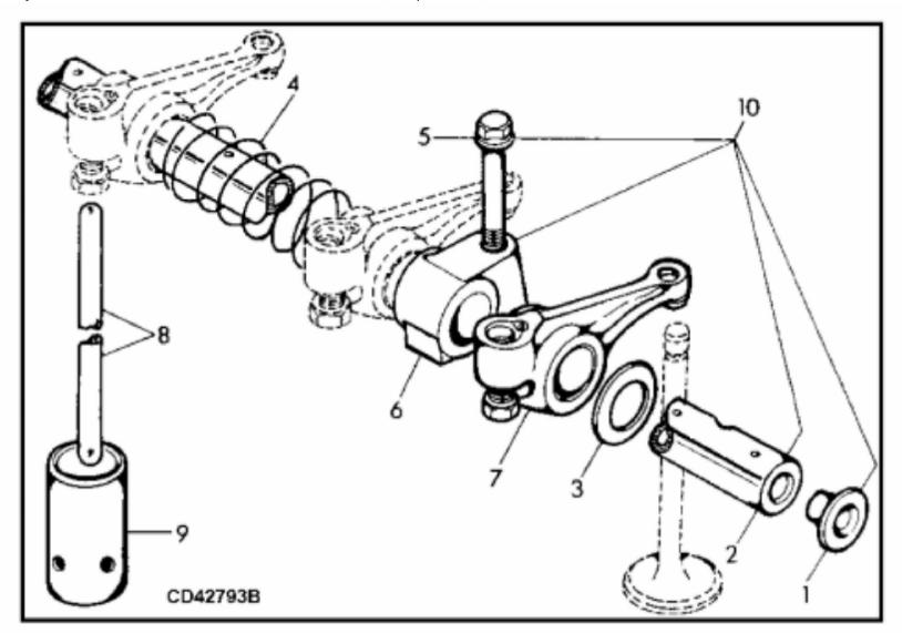
John Deere > Turf And Utility >TRACTOR >5510 - TRACTOR >5310, 5410, 5510 Tractors (Europe Edition) >20 ENGINE 3029DAT50 & 3029TAT50-DD16145 - DD16145 >ST116742 - ROCKER ARM SHAFT
