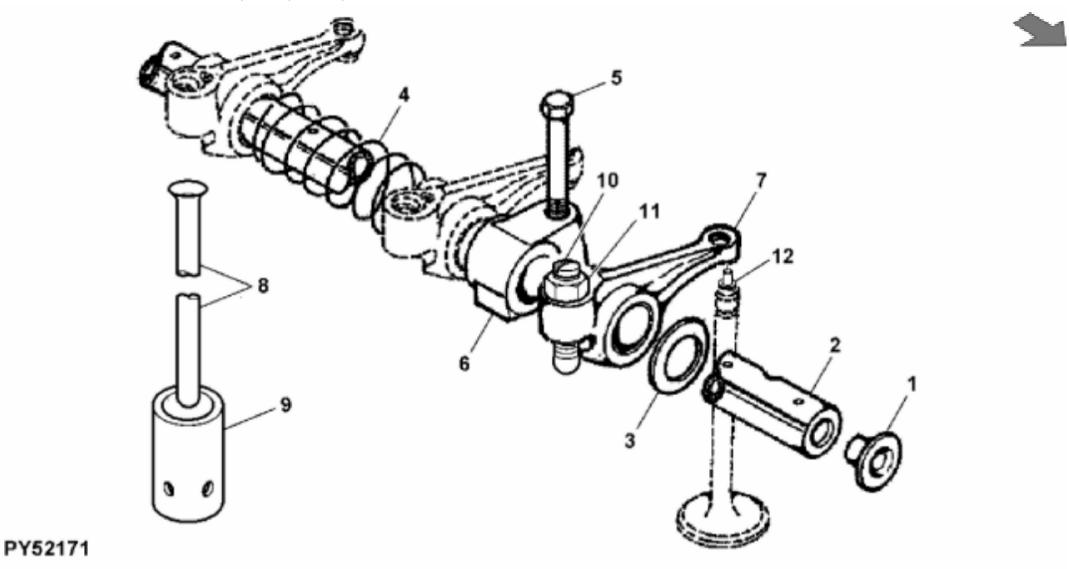
John Deere > Turf And Utility >TRACTOR >5075E - TRACTOR >5045D, 5045E, 5055D, 5055E, 5065E, 5075E Tractors (Tier 2)(8X4 and 9X3 TSS Transmission with OOS)(North America Edition) >20 ENGINE 3029TPY30-RE538148 >ST639677 - ROCKER ARM / SHAFT / TAPPET / PUSH ROD
