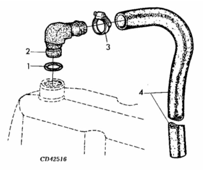
John Deere > Turf And Utility >TRACTOR >5075E - TRACTOR >5045D, 5045E, 5055D, 5055E, 5065E, 5075E Tractors (Tier 2)(8X4 and 9X3 TSS Transmission with OOS)(North America Edition) >20 ENGINE 3029TPY30-RE538148 >ST639675 - BREATHER
