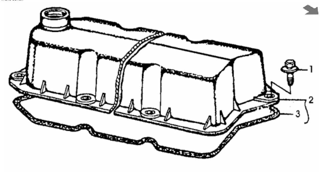
John Deere > Turf And Utility >TRACTOR >5075E - TRACTOR >5045D, 5045E, 5055D, 5055E, 5065E, 5075E Tractors (Tier2)(8X4 and 9X3 TSS Transmission)(Australia Edition) >20 ENGINE >ST639676 - VALVE COVER
