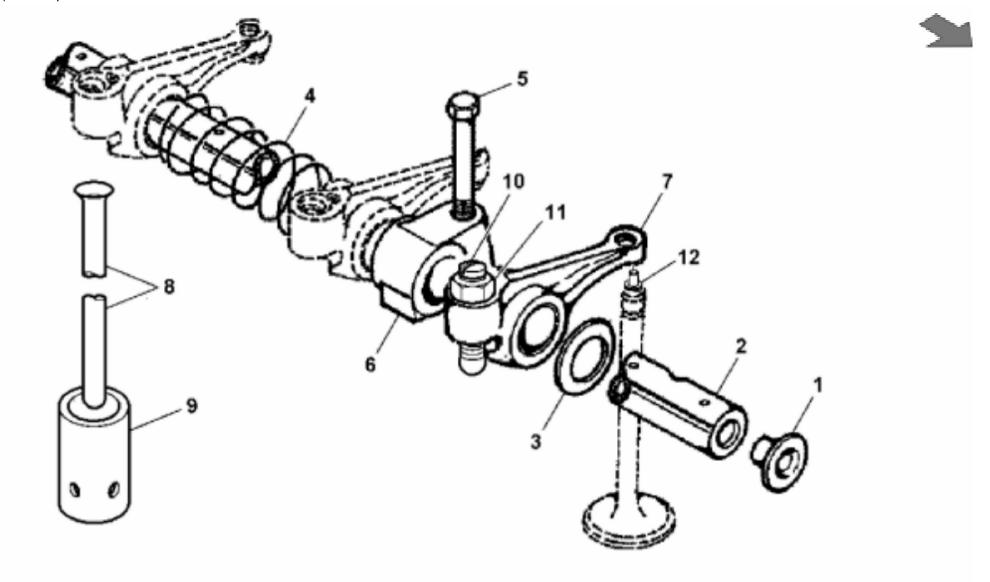
John Deere > Turf And Utility >TRACTOR >5075E - TRACTOR >5045D, 5045E, 5055D, 5055E, 5065E, 5075E Tractors (Tier2)(8X4 and 9X3 TSS Transmission)(Australia Edition) >20 ENGINE >ST639677 - ROCKER ARM / SHAFT / TAPPET / PUSH ROD
