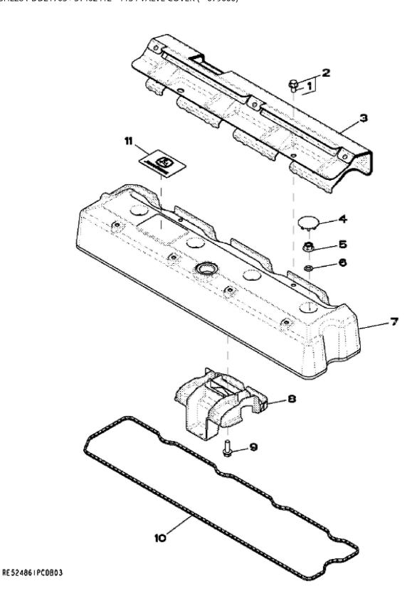
John Deere > Turf And Utility >TRACTOR >5080RN - TRACTOR >5080RN 5080RN Tractors (Europe Edition, Engine SN: CD4045LXXXXXXX) >24 ENGINE 4045HL284-DD21703 >ST402412 - 1134 VALVE COVER ( - 079666)
