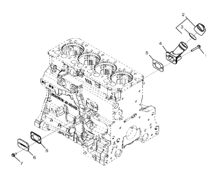
John Deere > Turf And Utility >TRACTOR >5090RN - TRACTOR >5090RN Tractors (Europe Edition, Engine SN: CD4045LXXXXXXX) >24 ENGINE 4045HL284-DD21703 >ST52635 - 1231 OIL FILLER NECK
