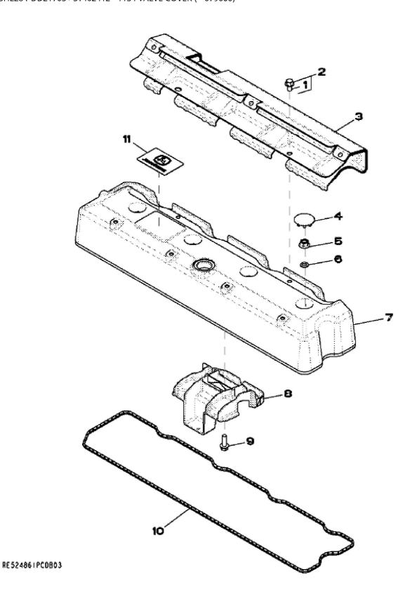
John Deere > Turf And Utility >TRACTOR >5090RN - TRACTOR >5090RN Tractors (Europe Edition, Engine SN: CD4045LXXXXXXX) >24 ENGINE 4045HL284-DD21703 >ST402412 - 1134 VALVE COVER ( - 079666)
