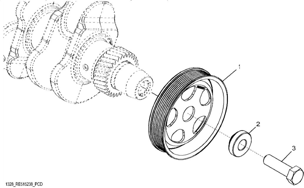
John Deere > Turf And Utility >TRACTOR >5080G - TRACTOR >5080G Tractor (Engine 4045HAT80)(Europe Edition) >20 ENGINE 4045HAT80-DD21692 >ST628039 - 1328 CRANKSHAFT PULLEY
