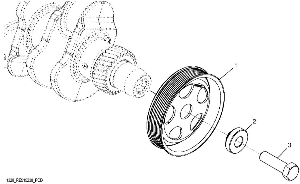
John Deere > Turf And Utility >TRACTOR >5090GH - TRACTOR >5090GH Tractor (Engine 4045HAT81)(Europe Edition) >24 ENGINE 4045HAT81-DD21693 >ST628039 - 1328 CRANKSHAFT PULLEY
