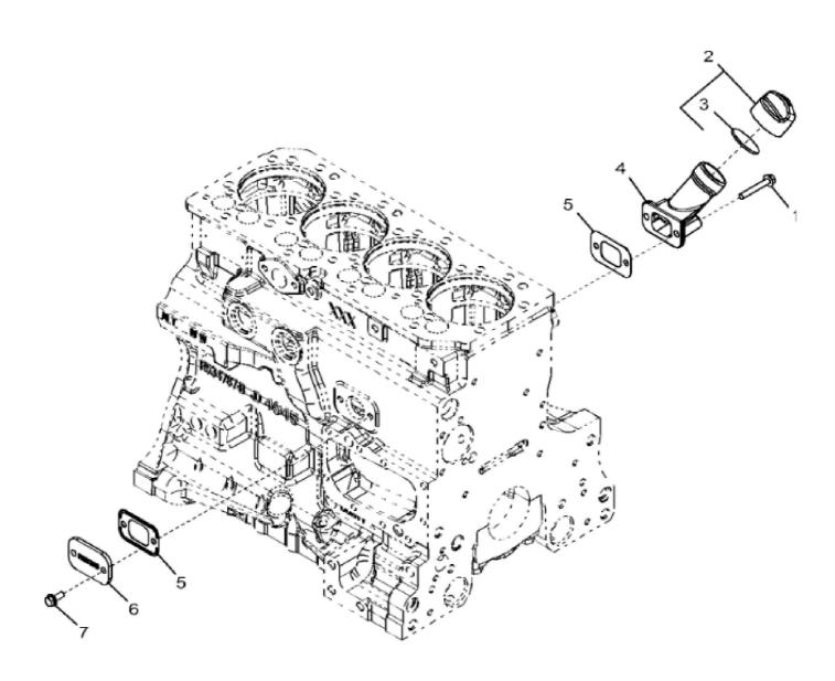
John Deere > Turf And Utility >TRACTOR >5090GH - TRACTOR >5090GH Tractor (Engine 4045HAT81)(Europe Edition) >24 ENGINE 4045HAT81-DD21693 >ST52635 - 1231 OIL FILLER NECK
