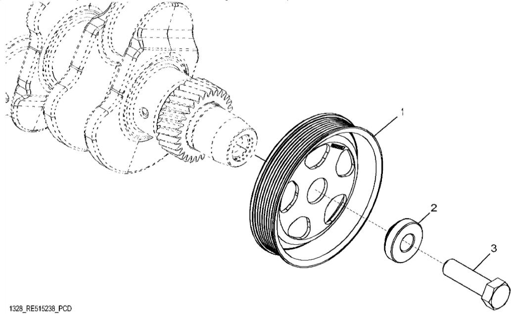
John Deere > Turf And Utility >TRACTOR >5080GF - TRACTOR >5080GF Tractor (Engine 4045HAT80)(Europe Edition) >24 ENGINE 4045HAT80-DD21692 >ST628039 - 1328 CRANKSHAFT PULLEY
