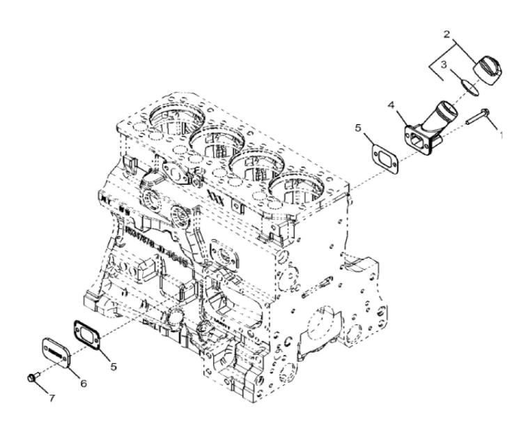
John Deere > Turf And Utility >TRACTOR >5090GF - TRACTOR >5090GF Tractor (Engine 4045HAT81)(Europe Edition) >24 ENGINE 4045HAT81-DD21693 >ST52635 - 1231 OIL FILLER NECK
