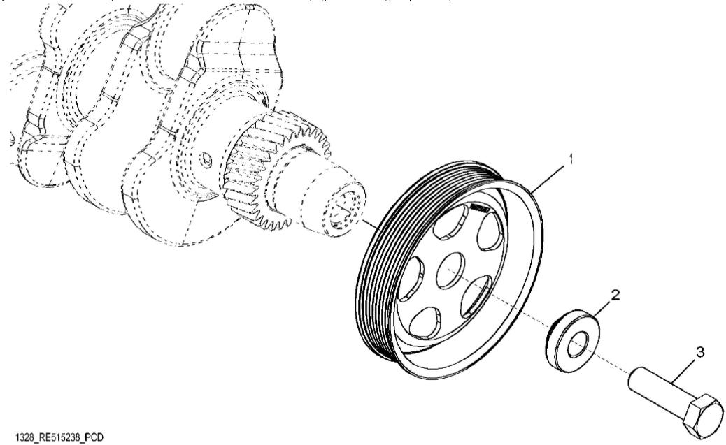
John Deere > Turf And Utility >TRACTOR >5090GV - TRACTOR >5090GV Tractor (Engine 4045HAT81)(Europe Edition) >24 ENGINE 4045HAT81-DD21693 >ST628039 - 1328 CRANKSHAFT PULLEY
